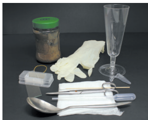
Apparatus used for the Baermann method
